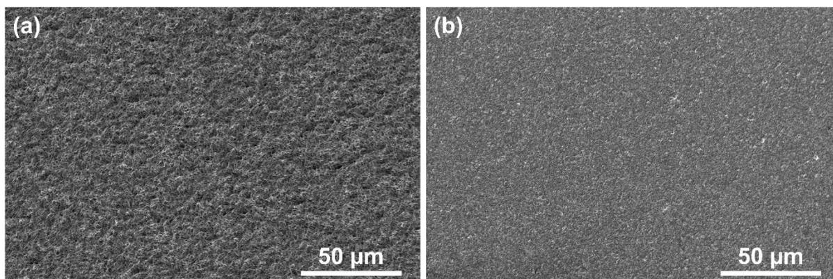
Figure S4. Surface Morphology of (a) In-doped ZnO and (b) pure ZnO film.
