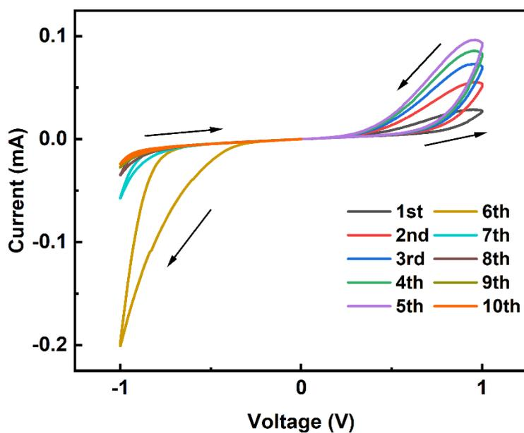
Figure S7. I-V curves of the ZnO-based device under 5 consecutive positive and 5 negative voltage sweeps.
