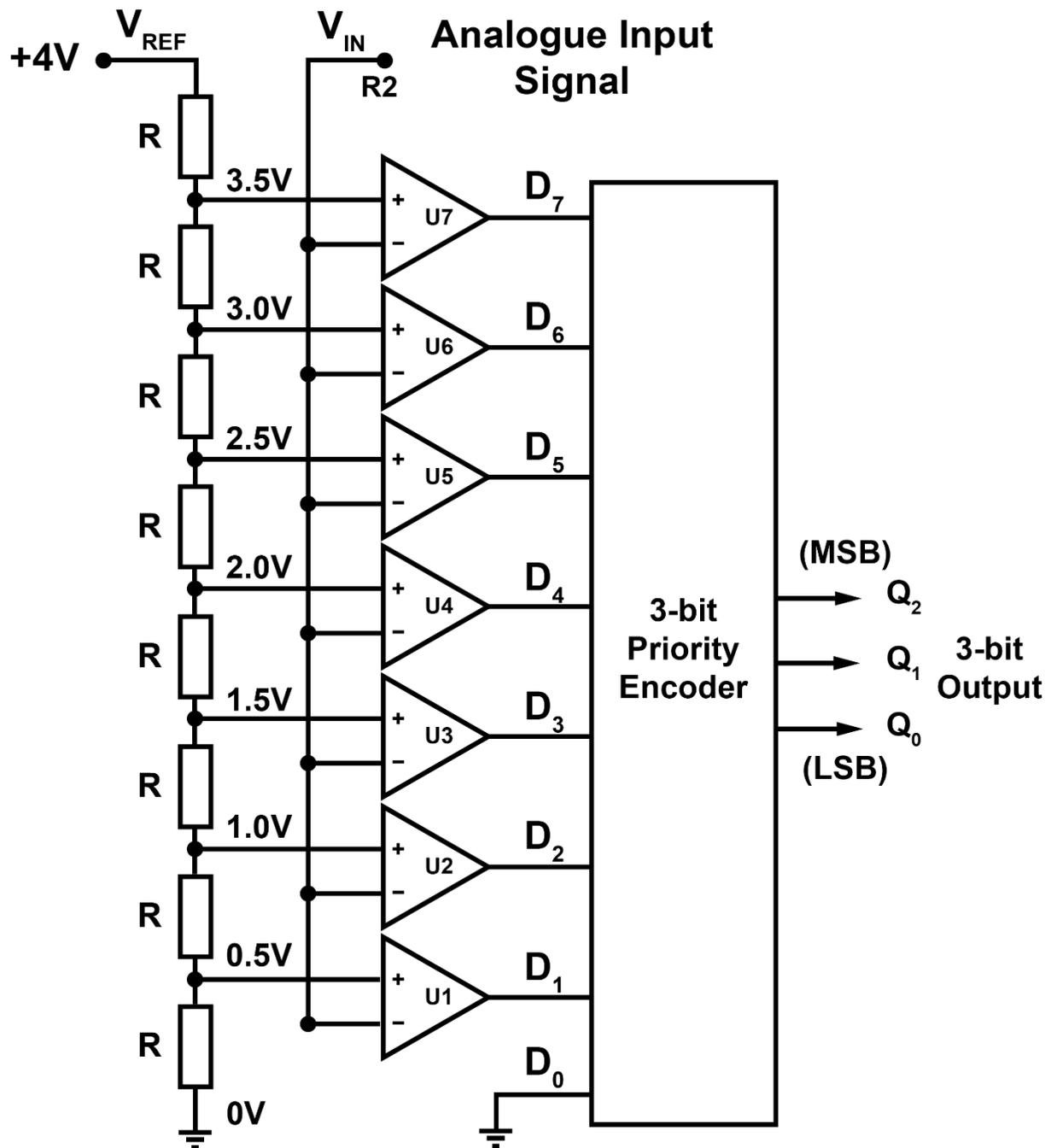
Figure S11. Circuit of analog to digital converter.<sup>[7]</sup>
