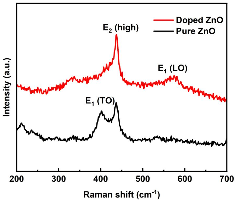
Figure S3. Raman results comparison of pure ZnO and In-doped ZnO film
