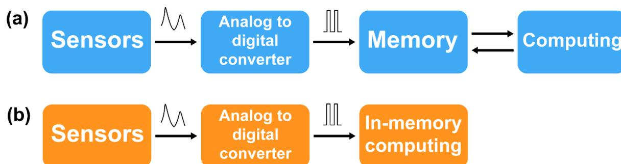
Figure S10. Schematic illustration of (a) Integrated sensor based on Von Neumann architecture (b) Integrated neuromorphic sensor.<sup>[1]</sup>
