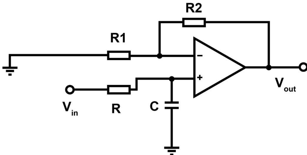
Figure S12. The First order low pass Butterworth filter.<sup>[7]</sup>
