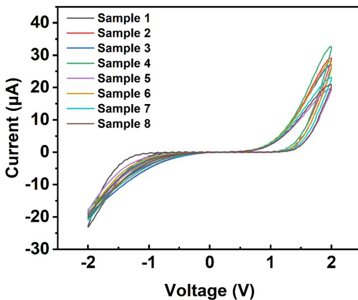
Figure S8. I-V curves of 8 different In-doped ZnO samples.
