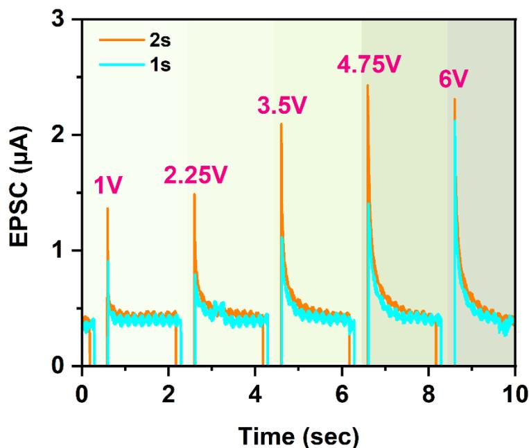
Figure S9. EPSC comparison under different pulse width (1s period)
