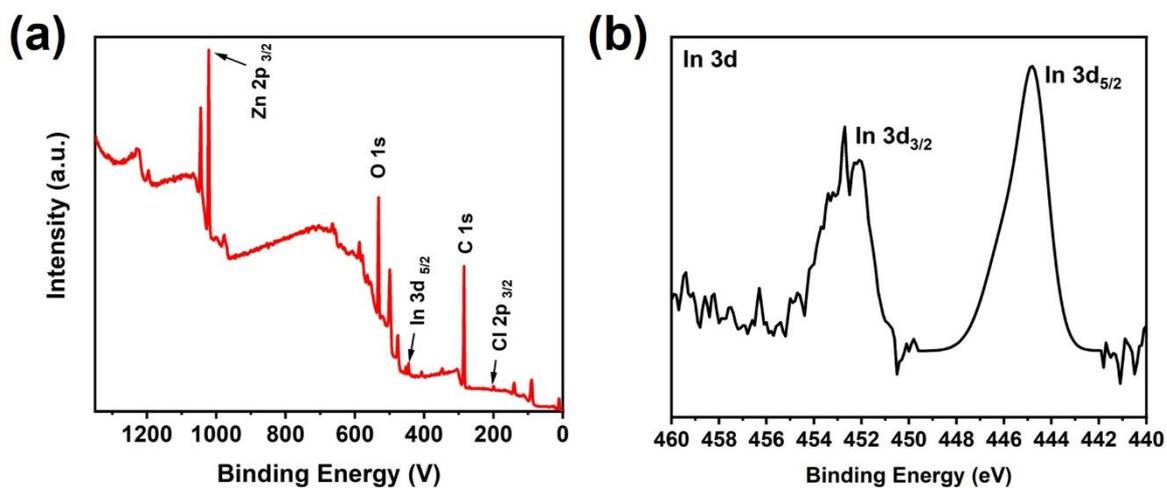
Figure S2. (a) XPS survey spectrum of ZnO:In film (b) XPS In 3d spectrum of ZnO:In film.
