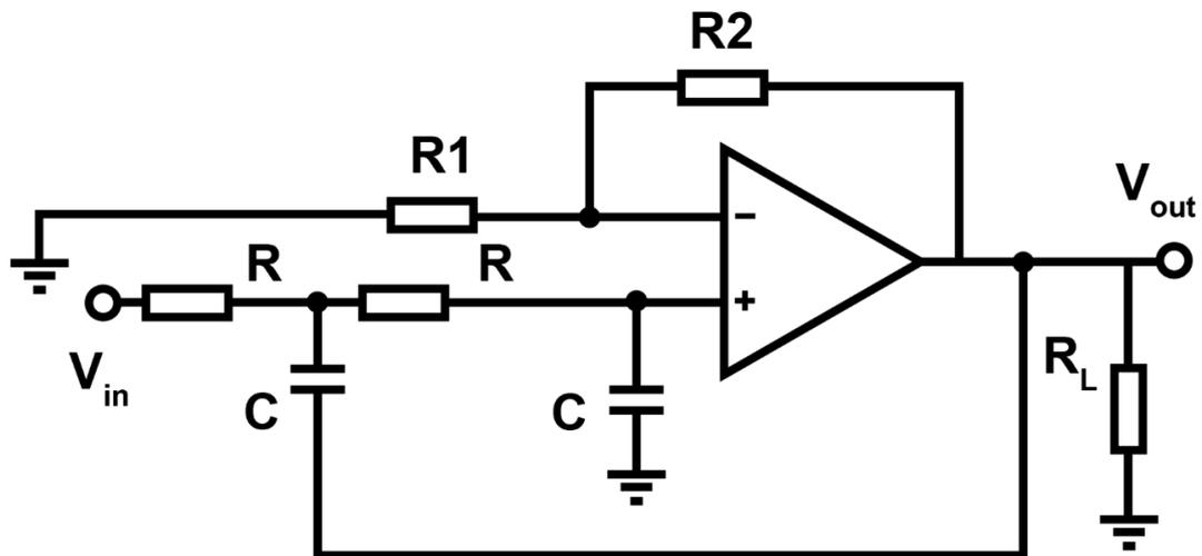
Figure S13. The second order low pass Butterworth filter.<sup>[7]</sup>
