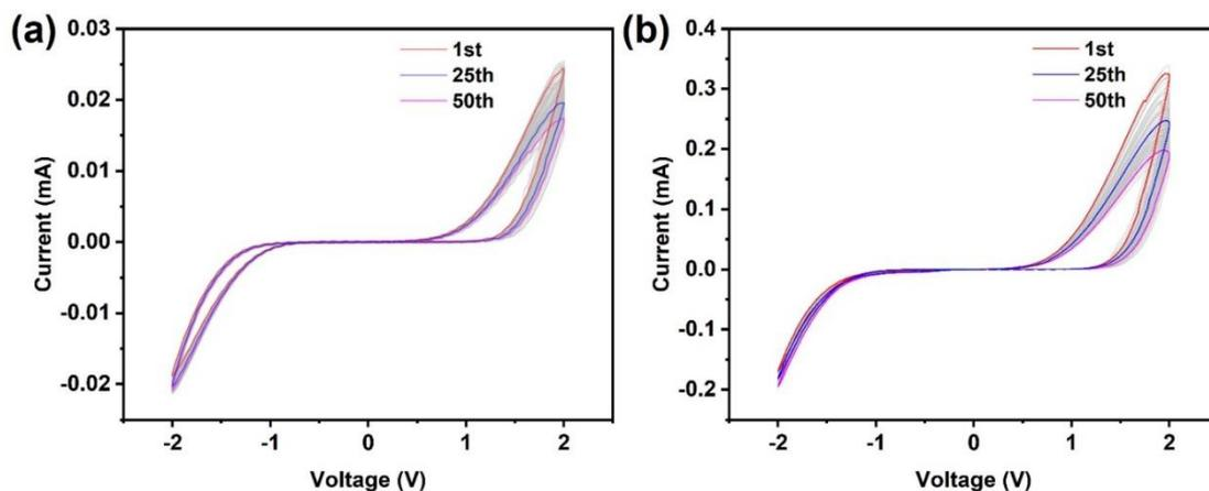
Figure S5. I-V curves under 50 positive and negative voltage sweeps ( $0\text{V} \rightarrow +2\text{V} \rightarrow 0\text{V} \rightarrow -2\text{V} \rightarrow 0\text{V}$ ): (a) In-doped ZnO and (b) pure ZnO film.
