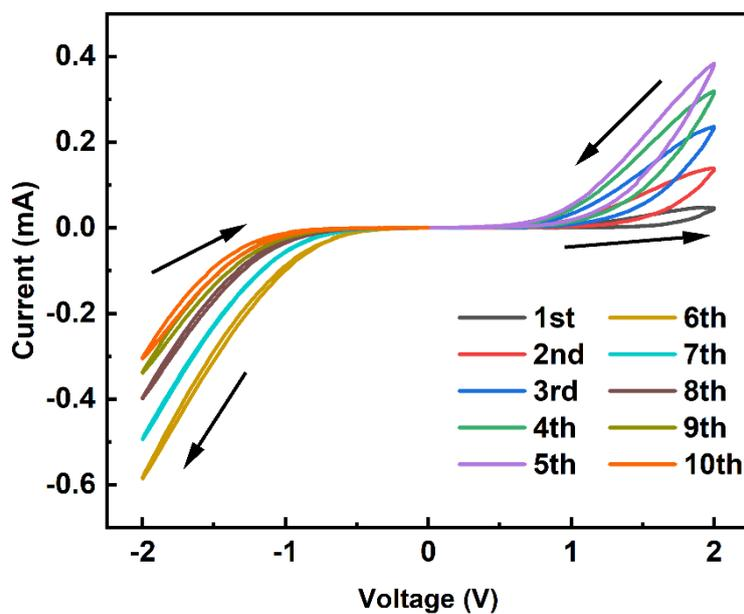
Figure S6. I-V curves of the In-doped ZnO-based device under 5 consecutive positive and 5 negative voltage sweeps.
